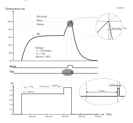
Figure 5.37: Example of the thermal model behaviour.
