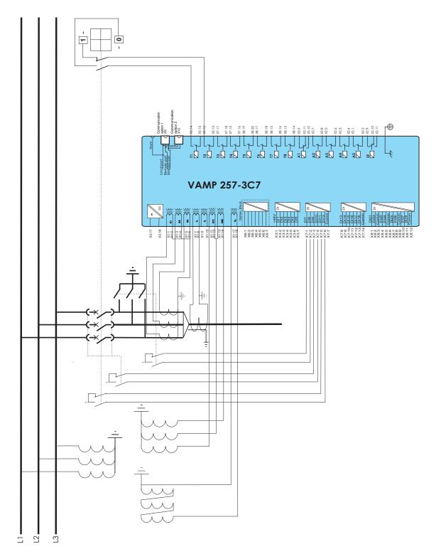
Figure 11.19: Connection example of VAMP 257-3C7. The voltage measurement mode is set to "2LL+ $U_0$ "
