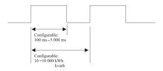
Figure 6.5: Principle of energy pulses
