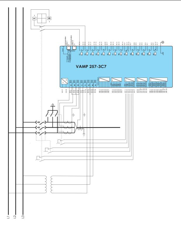
Figure 11.21: Connection example of VAMP 257-3C7 with V-connected voltage transformers. The voltage measurement is set to "2LL+ $U_0$ ". Directional earth fault stages are not available without the polarizing  $U_0$  voltage.
