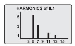
Figure 2.12: Example of harmonics bar display
