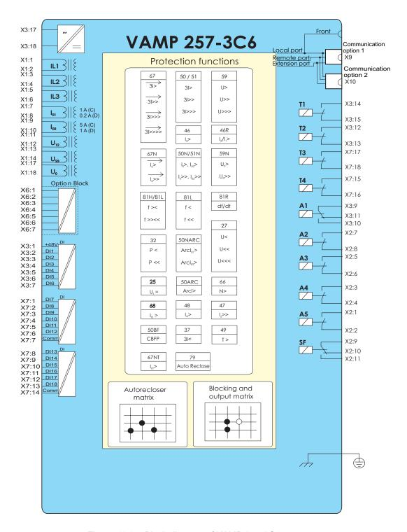
Figure 11.14: Block diagram of VAMP 257-3C6
