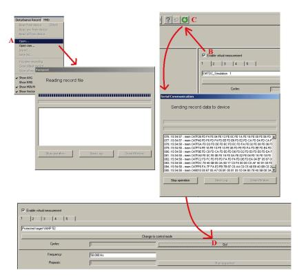
**NOTE:** The sample rate of the comtrade file has to be 32/cycle (625 micro seconds when 50 Hz is used). The channel names have to correspond to the channel names in VAMP relays:  $I_{L1}$ ,  $I_{L2}$ ,  $I_{L3}$ ,  $I_{01}$ ,  $I_{02}$ ,  $U_{12}$ ,  $U_{23}$ ,  $U_{L1}$ ,  $U_{L2}$ ,  $U_{L3}$  and  $U_{0}$ .
