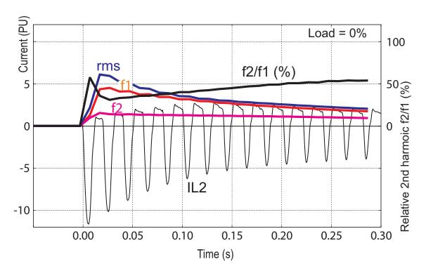
Figure 7.1: Example of various current values of a transformer inrush current
