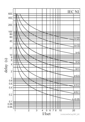
Figure 5.50: IEC normal inverse delay.
