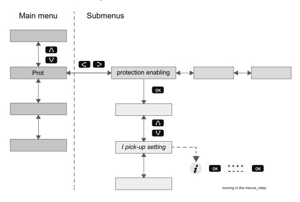
Figure 2.3: Moving in the menus using local HMI
