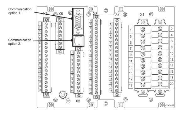
Figure 11.5: Example of VAMP 257 back panel serial communication connection
