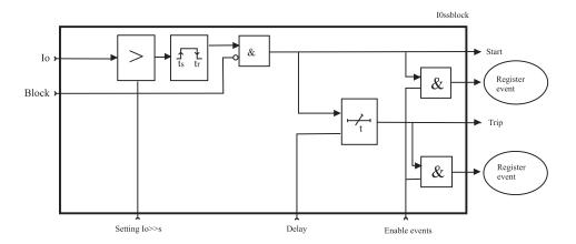
Figure 5.25: Block diagram of the earth fault stages  $I_0 >>, I_0 >>>>, I_0 >>>>$
