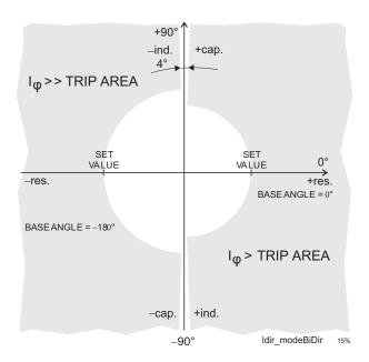
Figure 5.12: Bi-directional application with two stages  $I_{\varphi}$ > and  $I_{\varphi}$ >>.
