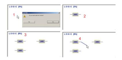
Figure 8.7: How to create logical nodes.
