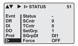
Figure 2.7: Example of protection submenu with setting group parameters
