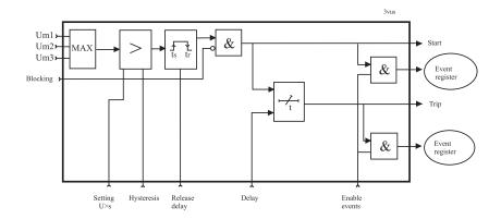
Figure 5.38: Block diagram of the three-phase overvoltage stages U>> and U>>>
