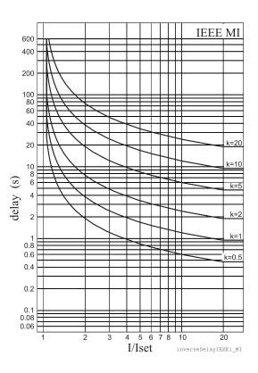
Figure 5.56: ANSI/IEEE long time extremely inverse Figure 5.57: ANSI/IEEE moderately inverse delay delay
