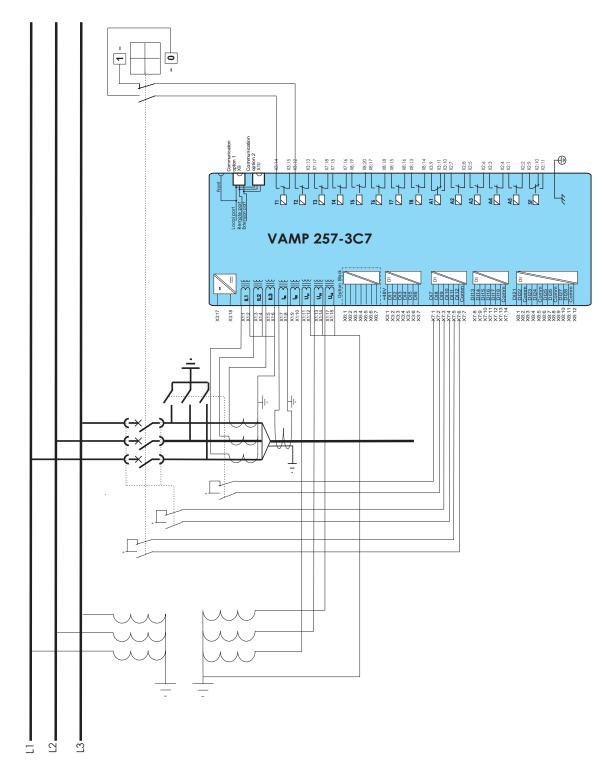
Figure 11.20: Connection example of VAMP 257-3C7 without a broken delta voltage transformer. The device is calculating the residual voltage. The voltage measurement mode is set to "3LN".
