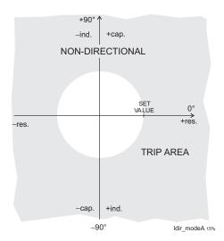
Figure 5.11: Difference between directional mode and non-directional mode. The grey area is the trip region.
