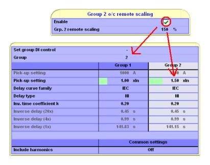
Figure 5.9: Remote scaling example.
