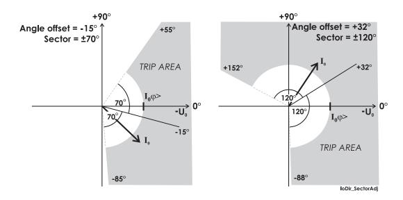
Figure 5.23: Two example of operation characteristics of the directional earth fault stages in sector mode. The drawn  $I_0$  phasor in both figures is inside the trip area. The angle offset and half sector size are user's parameters.
