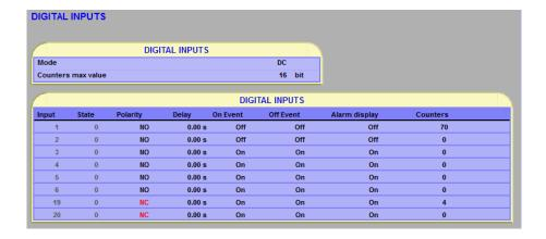
Figure 10.17: An example of digital input configuration for trip circuit supervision with two dry digital inputs DI19 and DI20
