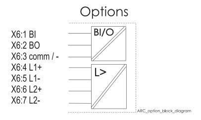
Figure 11.17: Block diagram of optional arc protection module.
