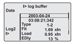
Figure 2.10: Example of selected fault log
