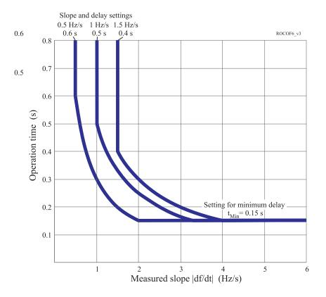
Figure 5.42: Three examples of possible inverse df/dt operation time characteristics. The slope and operation delay settings define the knee points on the left. A common setting for tMin has been used in these three examples. This minimum delay parameter defines the knee point positions on the right.
