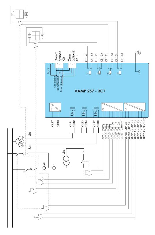
Figure 5.46: One synchrocheck stage needed with "1LL+U<sub>0</sub>/LLy "-mode.
