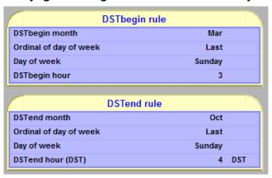
To ensure proper hands-free year-around operation, automatic daylight time adjustments must be configured using the "Enable DST" and not with the time zone offset option.
