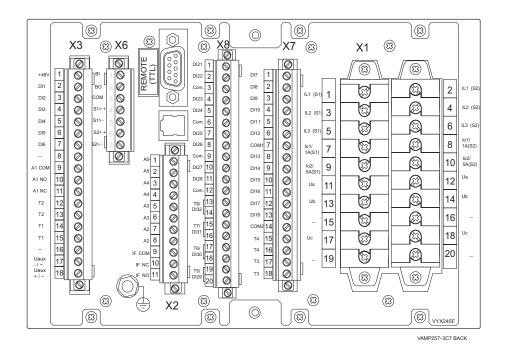
Figure 11.2: Connection on the rear panel of the VAMP 257-3C7
