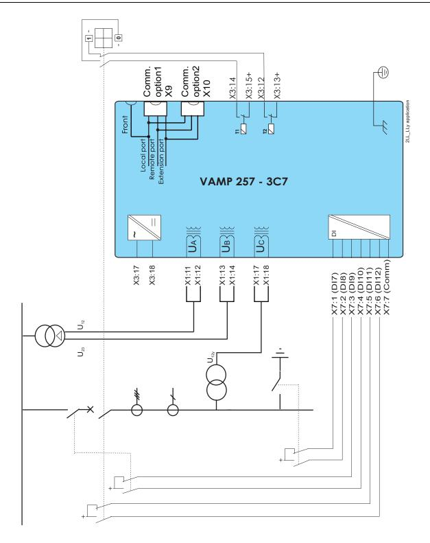
Figure 5.47: One synchrocheck stage needed with "2LL/LLy "-mode.
