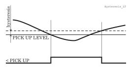
Figure 5.6: Behaviour of a less than comparator. For example in under-voltage and under frequency stages the hysteresis (dead band) acts according this figure.
