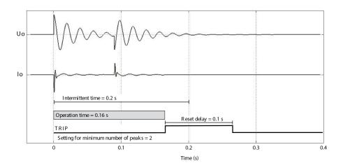
Figure 5.30: Set peak amount is satisfied and operation time comes full inside intermittent time setting. Stage issues a trip.
