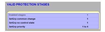
Figure 5.2: SetGrp priority setting is located in the Valid Protection stages view.
