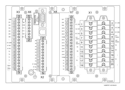
Figure 11.1: Connection on the rear panel of the VAMP 257-3C6
