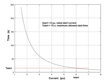
Figure 5.15: Example of an inverse operation time delay of the stall protection stage. If the measured current is less than the specified start current  $I_{START}$  the operation time will be longer than the specified start time  $T_{START}$  and vice versa.
