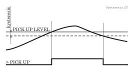
Figure 5.5: Behaviour of a greater than comparator. For example in overvoltage stages the hysteresis (dead band) acts according this figure.
