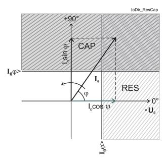
Figure 5.22: Operation characteristic of the directional earth fault protection in Res or Cap mode. Res mode can be used with compensated networks and Cap mode is used with ungrounded networks.
