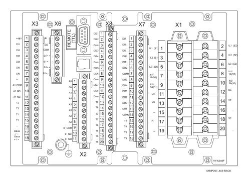
Figure 11.4: Connection on the rear panel of the VAMP 257-3C9
