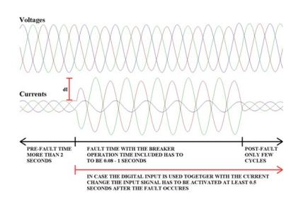
Below is presented an application example where the fault location algorithm is used at the feeder side. Notice following things while commissioning the relay:
