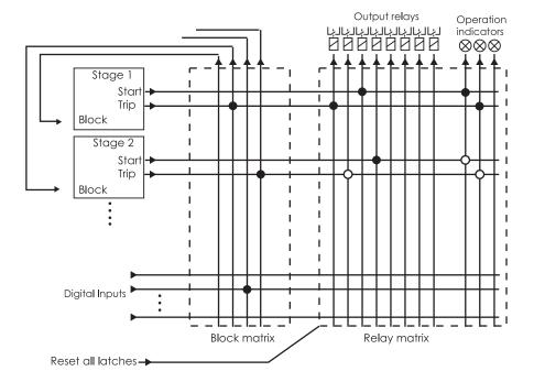
Figure 8.3: Blocking matrix and output matrix
