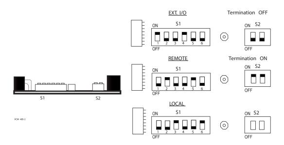
Figure 11.10: VCM 485-2- module's dip-switches
