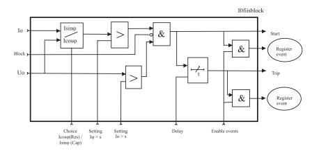
Figure 5.21: Block diagram of the directional earth fault stages  $I_{0\phi}$ >,  $I_{0\phi}$ >>,  $I_{0\phi}$ >>>
