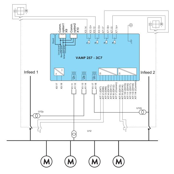
Figure 5.48: Two synchrocheck stages needed with "LL/LLy/LLz"-mode.
