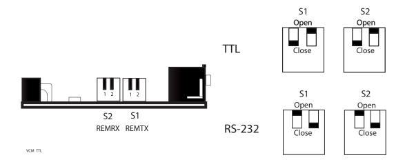
Figure 11.9: VCM TTL- module's dip-switches
