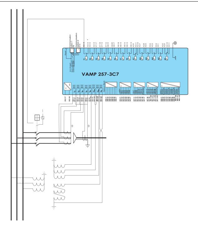
Figure 10.4: Example connection of VAMP 257. Both short circuits and earth-faults will be detected. The outgoing line is one of several parallel lines or the line is feeding a ring network.
