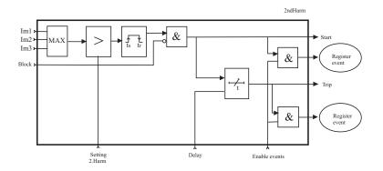
Figure 5.49: Block diagram of the magnetishing inrush stage.
