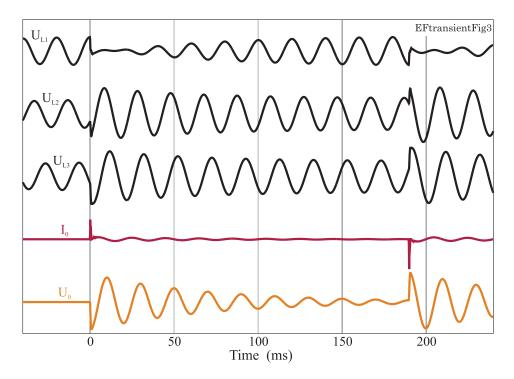
Figure 5.29: Typical phase to earth voltages, residual current of the faulty feeder and the zero sequence voltage  $U_0$  during two transient earth faults in phase L1. In this case the network is compensated.
