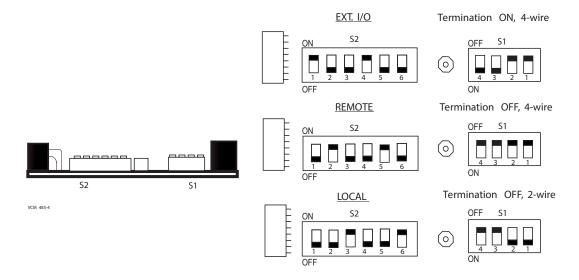
Figure 11.11: VCM 485-4- module's dip-switches
