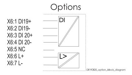
Figure 11.18: Block diagram of optional DI19/DI20 module with one arc channel.
