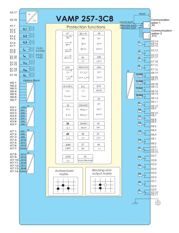
Figure 11.15: Block diagram of VAMP 257-3C8
