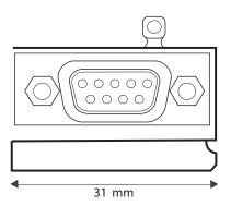
Figure 11.7: Communication module with a height of 31mm
