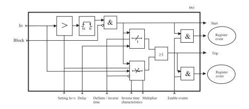
Figure 5.24: Block diagram of the earth fault stage I<sub>0</sub>>
