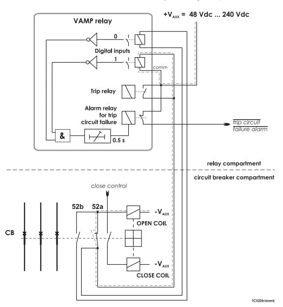
Figure 10.15: Trip circuit supervision with two digital inputs. The CB is closed. The supervised circuitry in this CB position is double-lined. The digital input is in active state when the trip circuit is complete. This is applicable for dry inputs only.
