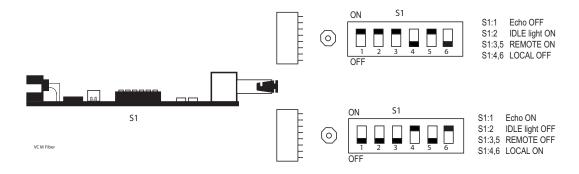
Figure 11.12: VCM Fiber- module's dip-switches
