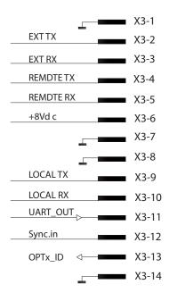
Figure 11.6: connection to communication modules
