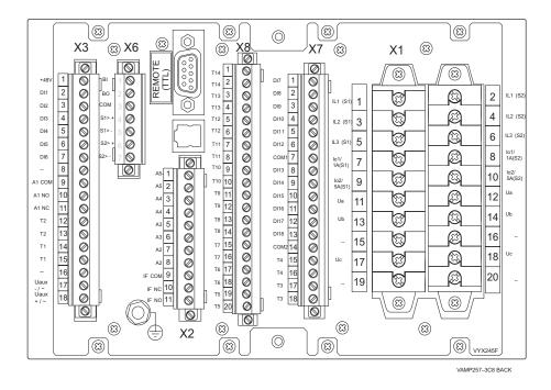
Figure 11.3: Connection on the rear panel of the VAMP 257-3C8
