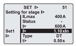
Figure 2.8: Example of I> setting submenu
