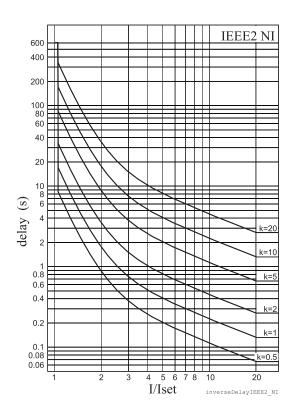
Figure 5.61: IEEE2 normal inverse delay
