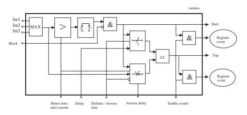
Figure 5.14: Block diagram of the stall protection stage  $I_{ST}$ >.
