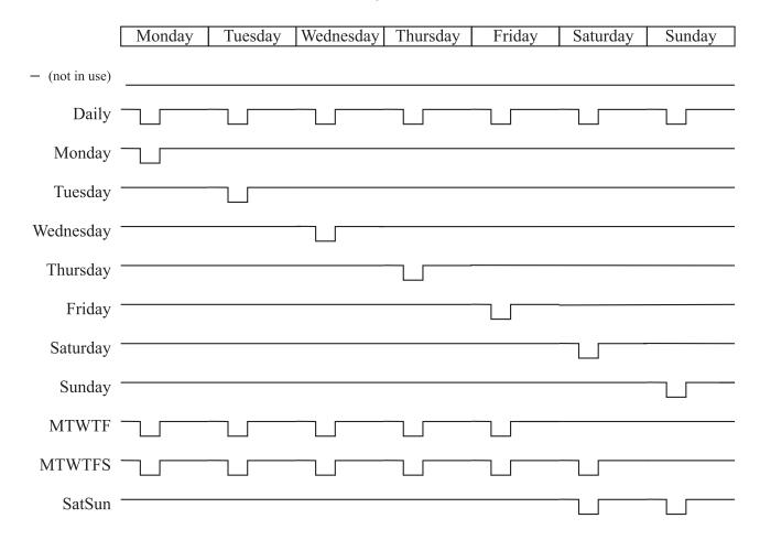
Figure 6.9: Timer output sequence in different modes.
