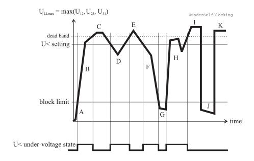
Figure 5.39: Under voltage state and block limit.
