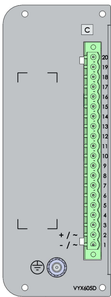
Figure 10.1: Example of supply voltage card Power C 110-240
