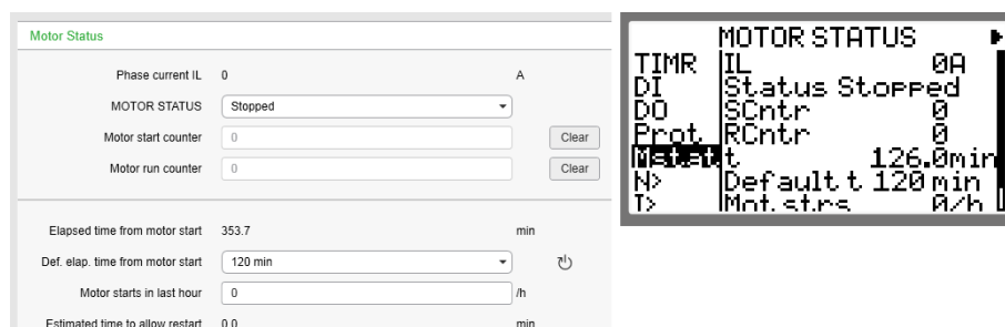
Figure 6.33: Motor status via Easergy Pro and local panel.
