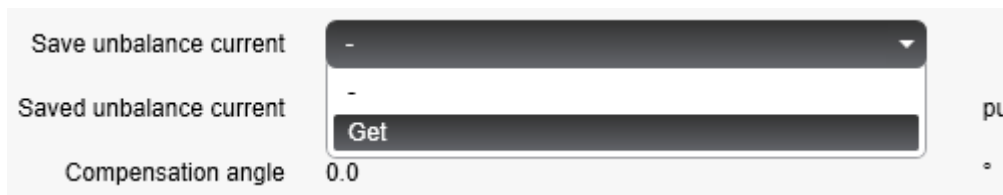
Figure 6.73: Saving the unbalance current
