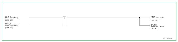
Fig. 3-52: Signals issued by measuring circuit monitoring
