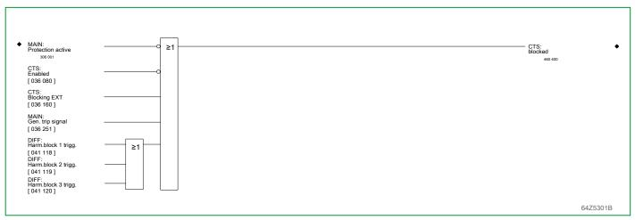
Fig. 3-120: Blocking of current transformer supervision
