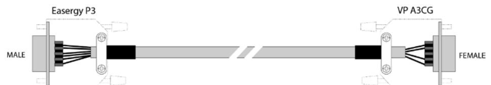
Figure 3.. Profibus cable REL52824 (VX072) for Easergy P3 Advanced
